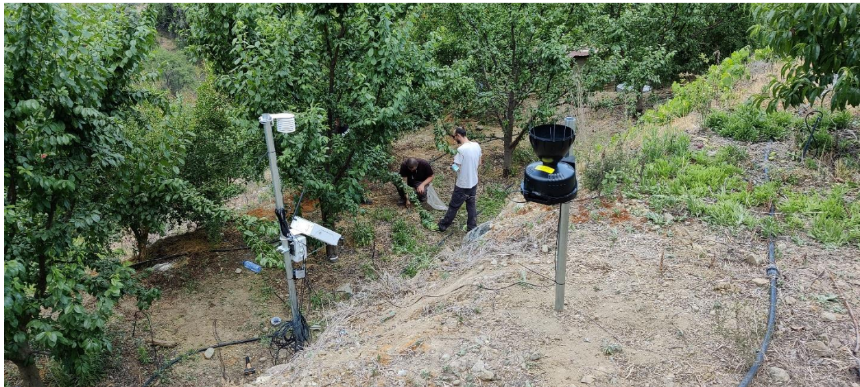
Figure 2: Establishment of soil moisture sensors and meteorological station in Dymes-Potamitissa plum orchard
